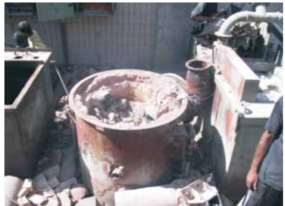
Cyanide salt annealing vessel with solidified chemicals
