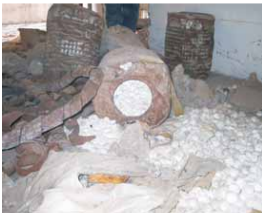
Degraded 300 litre barrels full of sodium cyanide pellets
