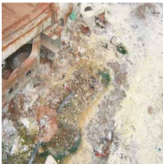
Surface soil contamination by metal compounds is clearly visible in parts of the site
